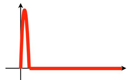
$$\begin{aligned} \dot{x}(t) &= Ax(t) + Bu(t) \\ y(t) &= Cx(t) \end{aligned} \quad \rightarrow \quad y_0(t) = Ce^{At}Bu_0$$
